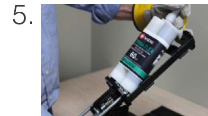
5. Place the cartridge in the spray gun
