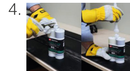
4. Remove the buckle and fasten the mixing tip
